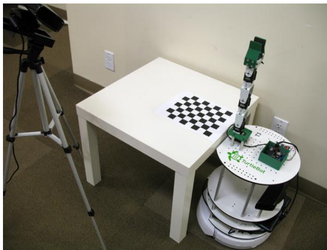
Fig. 3 Object placement and the working envelope of the robot arm [3]
